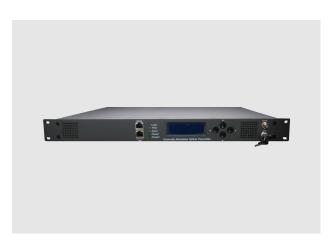
Build-in WDM, realizing the multiplex of main signal and inter-cut optical. The panel with main signal optical input port and join-wave output port can extra simplify the connection.
