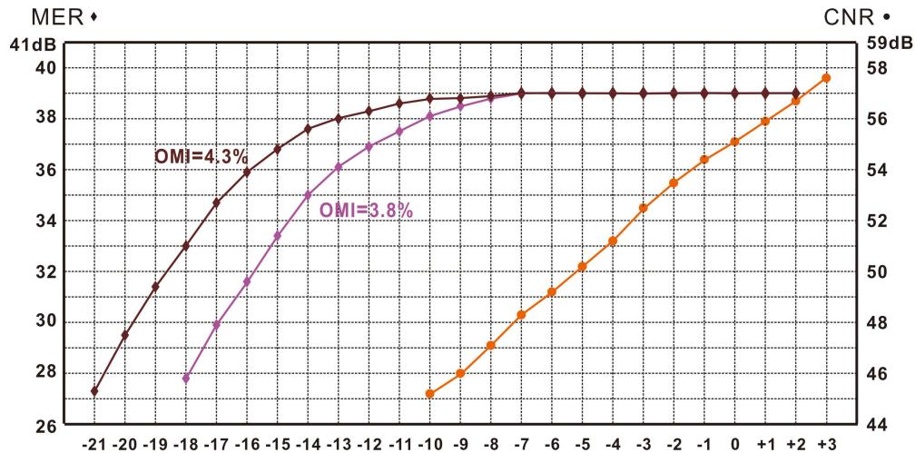
Note: 1. CNR Test conditions: 59CH PAL-D, OMI = 3.8%
