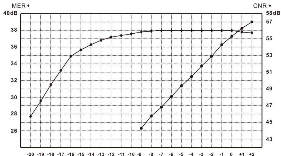
Note: 1. CNR test condition: 59CH PAL-D, OMI=3.8%
