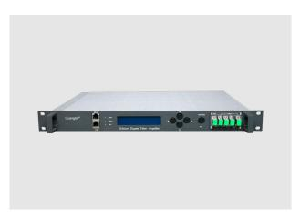
HA5700, the Mid-Stage Access (MSA) CATV fiber amplifier, is developed and produced specially for the dispersion compensation of over-long trunk. HA5700 is composed of lower noise per-amplifier (PA) and booster amplifier (BA). There is access connector between these two amplifiers and thus the dispersion compensation module (DCM) can be accessed in the mid-stage conveniently. It offers the most simple and effective application.
