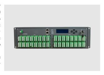
HA5800C has extremely low noise figure, the entire unit adopts twin-stage amplification, and the pre-amplifier adopts low noise EDFA, output cascade adopts high power EYDFA. When input optical power Pin=0dBm, the noise figure of unit is ≤5.5dB Unlike other kind of product which need high optical power input to maintain lower noise figure.
