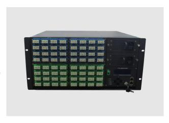
HA5800E has extremely low noise figure, the entire unit adopts twin-stage amplification, and the pre-amplifier adopts low noise EDFA, output cascade adopts high power EYDFA. When input optical power Pin=0dBm, the noise figure of unit is ≤5.5dB Unlike other kind of product which need high optical power input to maintain lower noise figure.
