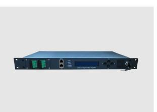
greatly reduces the overall thermal power, to ensure long life and high reliability PUMP Laser work. Front panel LCD, LED offers the work parameters and alarms. RS232 and RJ45 provides serial communications and SNMP network management interface. Optical loss, laser automatically shut down, provides laser safety protection.
