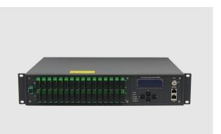
HA5800B has extremely low noise figure, the entire unit adopts twin-stage amplification, and the pre-amplifier adopts low noise EDFA, output cascade adopts high power EYDFA. When input optical power Pin=0dBm, the noise figure of unit is <5.5dB Unlike other kind of product which need high optical power input to maintain lower noise figure.
