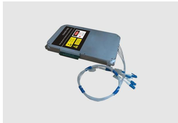
variable gain booster amplifier (BA). The gain of these two stages amplifier can be independently set in a certain range. There is a connector between the two stages amplifier, which used for mid-stage access, such as optical Add-Drop module (OADM), dispersion compensation module (DCM) and others optical modules.
