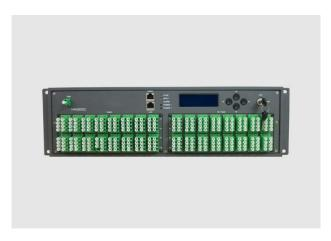
HA5800C has extremely low noise figure, the entire unit adopts twin-stage amplification, and the pre-amplifier adopts low noise EDFA, output cascade adopts high power EYDFA. When input optical power Pin=0dBm, the noise figure of unit is ≤5.5dB Unlike other kind of product which need high optical power input to maintain lower noise figure.
