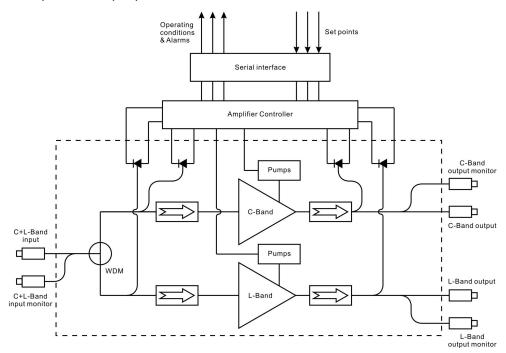
2.Optical port mode 11 (1×C+L-Band input, 1×C+L-Band output. With input & output monitor port)
